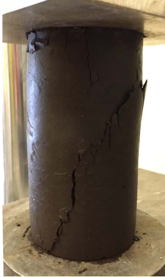
Figure 3.7 Unconfined compression testing of 3 x 6 in. cylinders.
