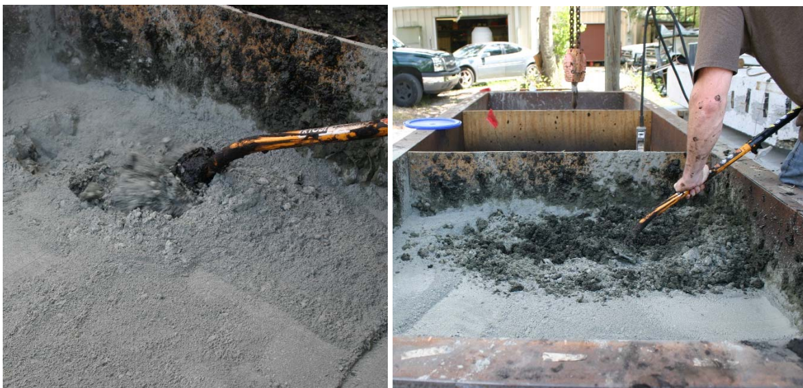
Figure 4.30 Dry mixing progression, part 1 of 2.
