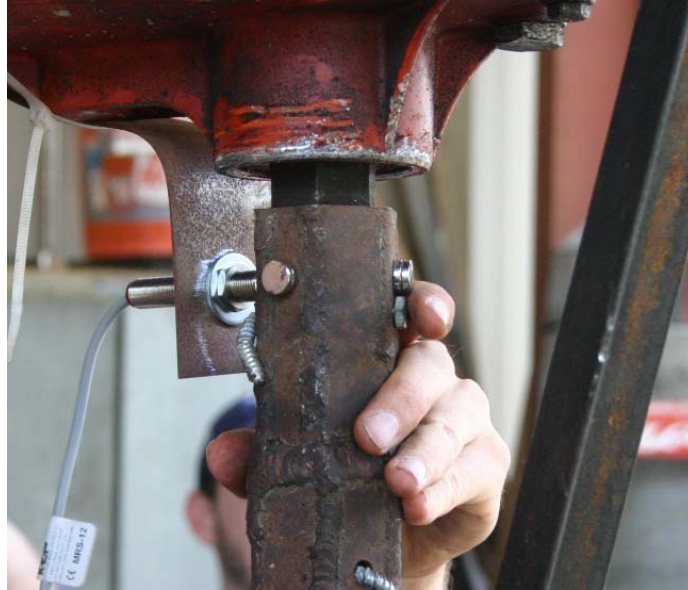
Figure 4.8 Magnetic rotation counter.
