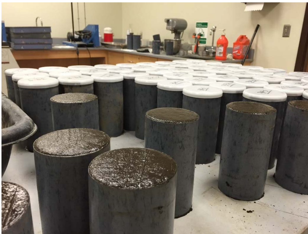
Figure 3.6 Prepared 3 x 6 in. cylinders.
