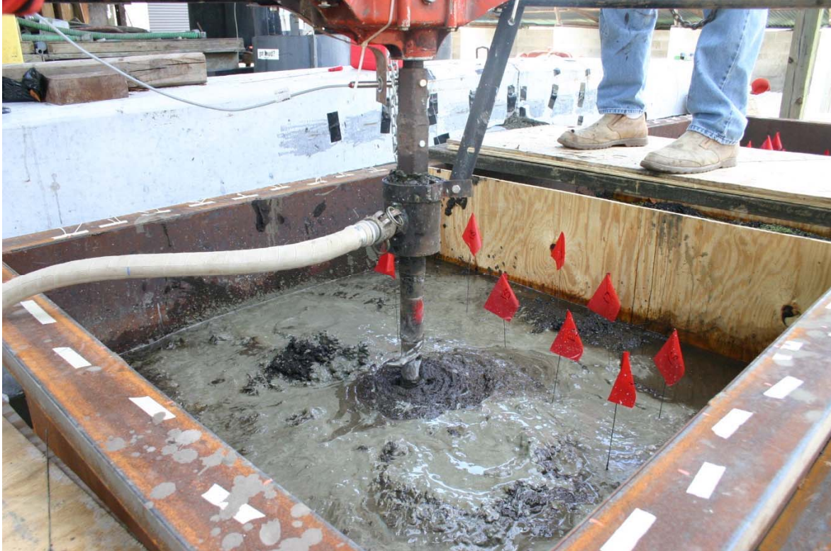
Figure 4.24 Close up of wet mixing.
