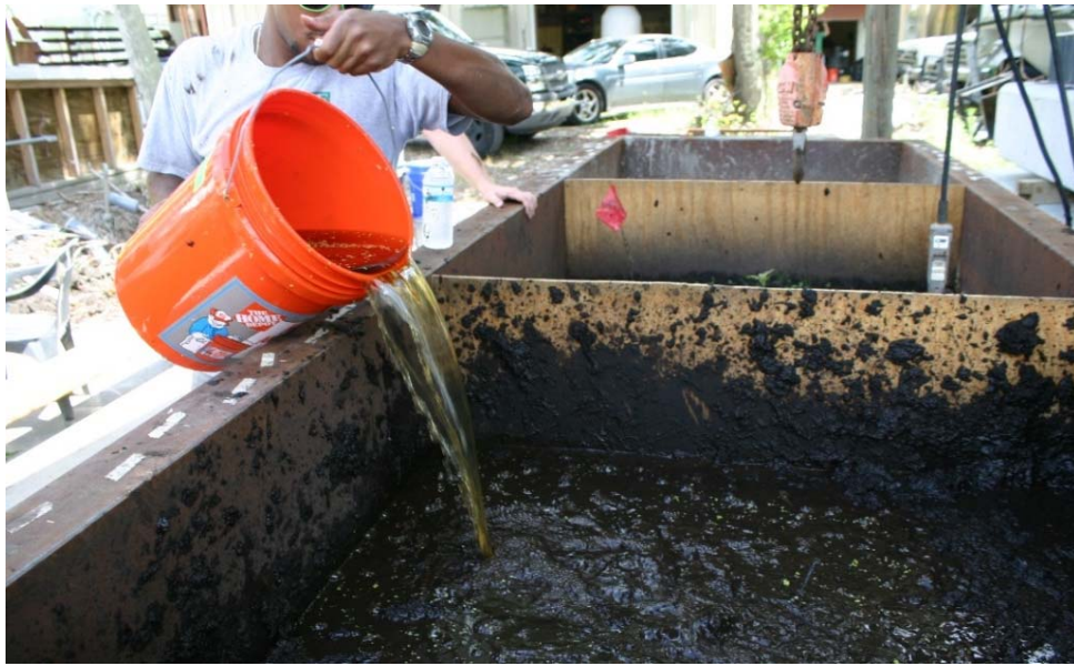
Figure 4.26 Rainwater added to maintain saturation condition.
