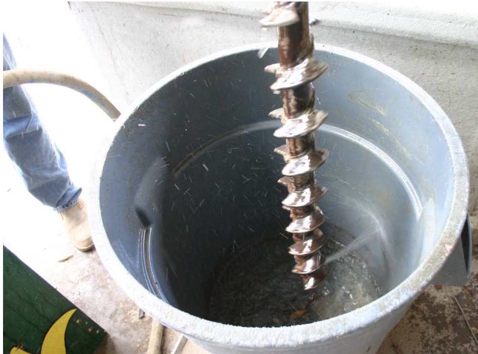
Figure 4.11 Modified auger in test barrel.
