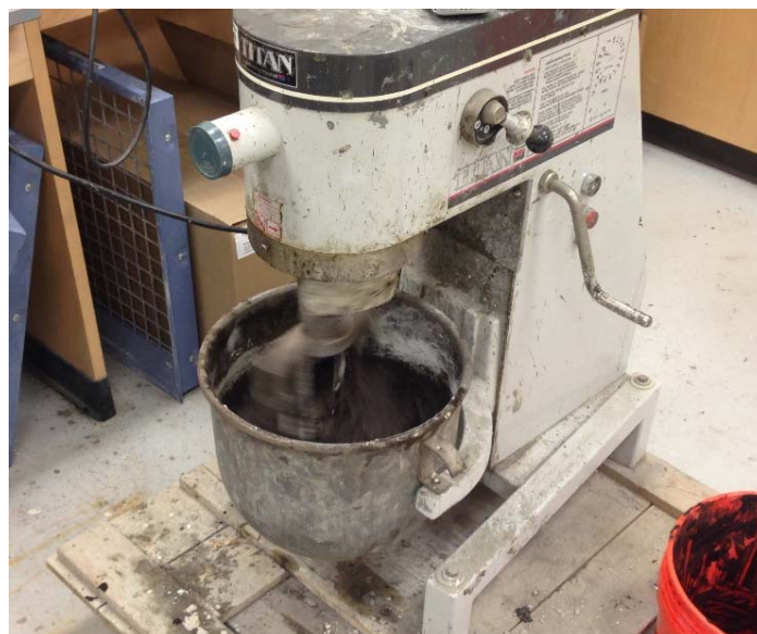
Figure 3.5 Small scale laboratory mixer.
